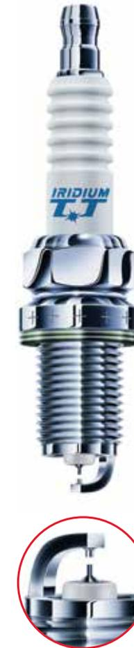
Nickel Plugs feature two flat surfaces, which block the ability of the ignition spark to grow. But DENSO's Iridium TT's two needle-thin electrodes (with the center electrode 0.2mm smaller than the nearest rival) act as thinner 'fingers', allowing the spark to expand 360 degrees in all 3 dimensions.
